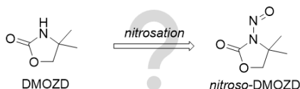
Scheme 3: A more unlikely, but possible nitrosamine that could form during CESAR1 degradation.
